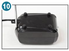
10. Re-install bottom of main housing and secure with four screws.
