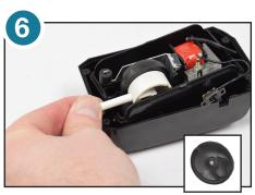
6. Remove diaphragm assembly from unit. Inspect magnets and clean if needed. Remove and save the black seal shown in the inset photo. This is not included in this repair kit. You will use this in step 7.
