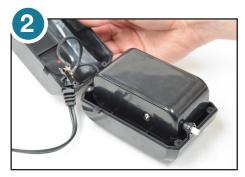
2. Carefully lift top of housing back to access internal housing.
