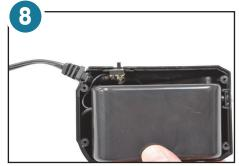
8. Arrange electrical cords in slot and press lid back onto internal housing.
