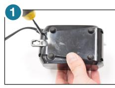
1. Unplug unit and remove four screws from bottom housing.
