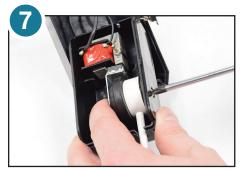
7. Press the black seal into the side of the new diaphragm assembly Install new diaphragm assembly by holding it securely to the side while tightening screw.
