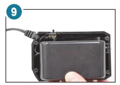
9. Place internal housing back into top of main housing. Arrange cords and switch to avoid pinching when reassembling main housing.
