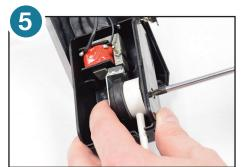
5. With lid off, remove screw from side of housing that holds diaphragm assembly in place.
