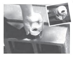
Thread the 2" male adapter into one of the ports on the filter using teflon tape or silicone on the threads.
