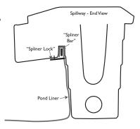
sible. The liner should be run up the stream or to the filter box. Folder the liner over the Spliner Lock. Slide the Spliner Bar into the spline channel and secure with the Spliner Locks. Be sure
