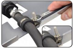
Use washer on both sides of base. Insert 10mm bolt from bottom side and tighten nut to clamp down tubing and provide strain relief.
