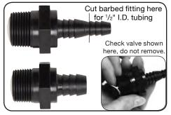
3/4" MPT barbed check valve is designed to be used with 1/2" or 3/8" I.D. tubing. Use larger barbed fitting for 5/8" ID tubing
