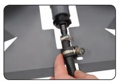
Fit padded hose clamp over tubing. (Use 17.5mm clamp for <sup>3</sup>/<sub>8</sub>" tubing or 25.5mm clamp for <sup>1</sup>/<sub>2</sub>" and <sup>5</sup>/<sub>8</sub>" tubing)
