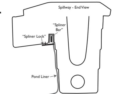
Folder the liner over the Spliner Lock. Slide the Spliner Bar into the spline channel and secure with the Spliner Locks. Be sure
