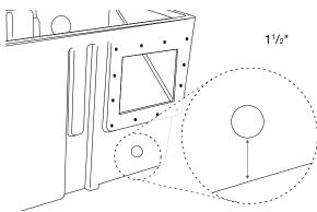
You will need to cut a hole into the front of the skimmer box.  $3^{\circ}$  for BDK2 or  $4^{5}/8^{\circ}$  for BDK3. Hole is usually centered from left to right and bottom of hole is approximately  $1^{1}/2^{\circ}$  up from bottom of skimmer.
