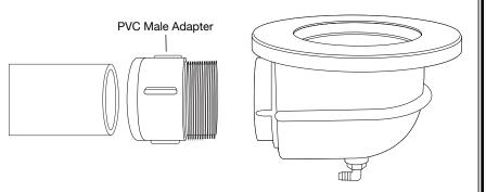
prior to glueing bottom drain to PVC pipe. Failure to clamp securely could result in leaking. Extend tubing out beyond edge of liner to be connected to air pump. Be sure air compressor sits higher than water level in pond after tubing is connected. Recommended air flow is 0.5 - 1.5 cfm.
