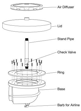
■ Drain base is installed under the liner, usually in the deepest part of the pond. Determine placement and excavate. Bottom drain and plumbing use a PVC 4" male adapter or reducing adapter to connect to PVC pipe (not included). Teflon tape threads of male adapter and tighten securely to prevent leaking. Connect ¹/₂" tubing to barbed elbow (installed) and clamp securely prior to glueing bottom drain to PVC pipe
