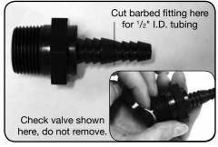
1.  $^{3}/_{4}$ " MPT barbed check valve is designed to be used with  $^{1}/_{2}$ " and  $^{3}/_{8}$ " I.D. tubing. Remove end of barb if installing  $^{1}/_{2}$ " I.D. tubing.
