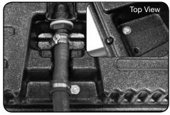
6. Use washer on both sides of base. Insert 10mm bolt and tighten nut to clamp down tubing and provide strain relief.
