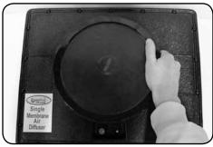
8. Screw diffuser(s) onto <sup>3</sup>/<sub>4</sub>" FPT on top of unit. Snug fitting by hand, do not overtighten.
