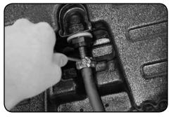
4. Slide hose clamp back over tubing and fasten with regular screwdriver or nut driver.
