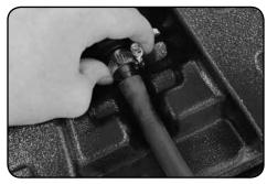
3. Slip hose clamp over barbed check valve and push tubing tightly onto the fitting.
