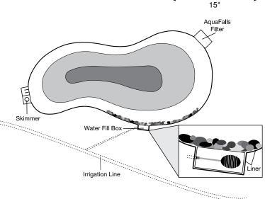
as the top of the pump. This way if the water level drops, the autofill will add water and protect the pump.
