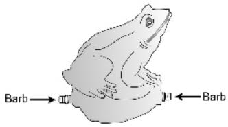
3. Cut and size hose, connect to the Statuary UV and the pump with hose clamps do not over tighten. Keep this run as short as possible to avoid kinks or bends. The pump should be as far away from the Statuary UV as possible for optimal water circulation. Keep in mind the length and run of the needed hose when purchasing, measuring and cutting.
