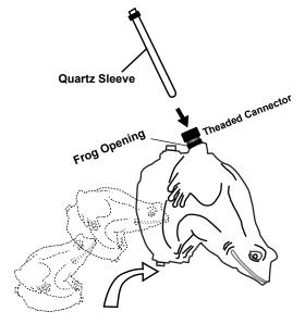
10. Push the Rubber Seal into the UV until it touches the inner rim of the Threaded Connector. The Rubber Seal should be 1/4" from the end of the Quartz Sleeve 1/2 of the Rubber Seal should be visible.
