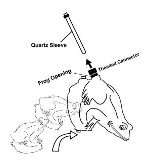
8. Once the Quartz Sleeve is removed it can be cleaned with Lime Away or similar products.
