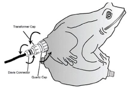
5. Slide the Lamp out of the Statuary Body. An angle, even a slight angle may cause a "U" shaped crack at the end of the Quartz Sleeve, or possible breakage of the Lamp. If this should happen, do not proceed with the installation. Purchase a new Quartz Sleeve or Lamp from your dealer. Do not force the Lamp out of the Quartz Sleeve; any force would be an indication of an improper removal.
