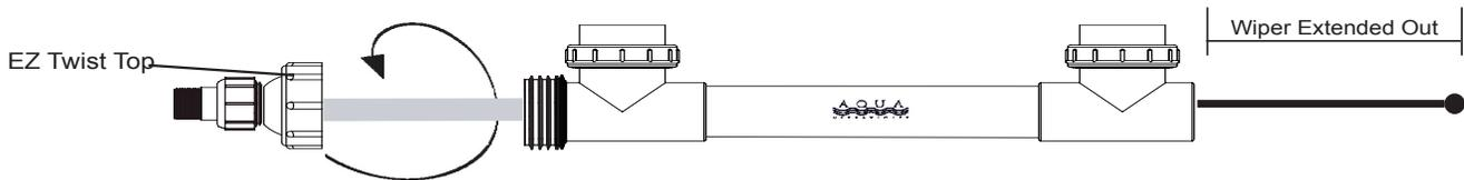
8. Remove the Quartz Sleeve Assembly.
