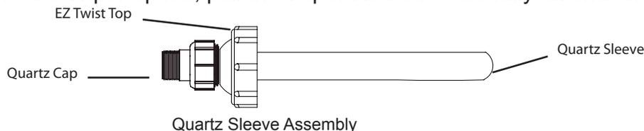
2. Untwist E-Z Twist Top. This will release the Quartz Sleeve Assembly. Pull The Quartz Sleeve Assembly straight out of the housing.
