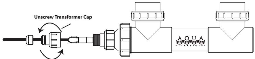
4. Slide Lamp out, be careful not to slide the Lamp out at an angle, even a slight angle, this may cause a "U" shaped crack at the opening of the Quartz Sleeve, or possible breakage of the Lamp. A Broken Lamp or Quartz Sleeve are not covered under warranty.
