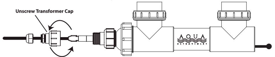
4. Slide Lamp out, be careful not to slide the Lamp out at an angle, even a slight angle, this may cause a "U" shaped crack at the end of the Quartz Sleeve, or possible breakage of the Lamp. Set the lamp on a secure level surface to avoid breakage.
