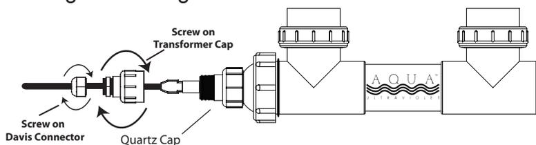
5. Tighten the Davis Connector back on to the Transformer Cap.
