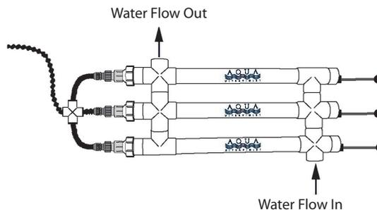
Plumb the water going in from the bottom and out through the top. This will help ensure the chamber stays full of water.
