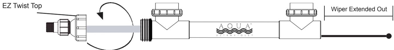
5. Pull the Wiper Rod completely out (fully extended)
