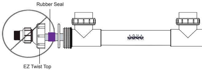
Incorrect: Quartz Sleeve is Outside of Wiper Blade
