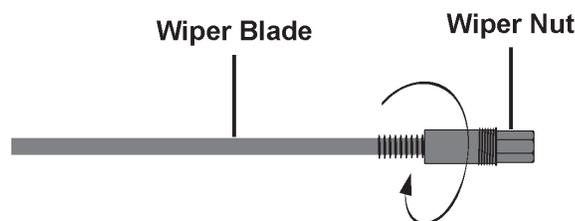
17. Using a 1/2" wrench screw the nut into the base of the unit. Be careful not to cross thread.
