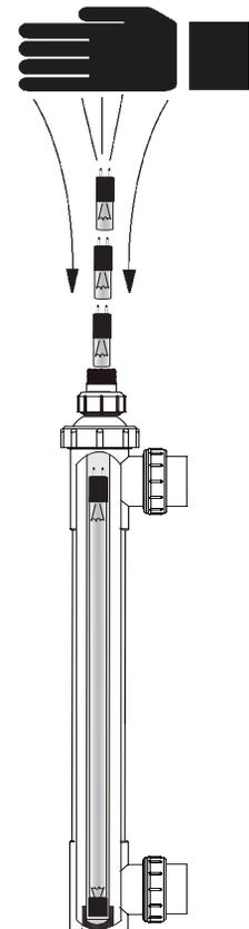
Incorrect: Lamp at an Angle will create a U Shaped Crack
