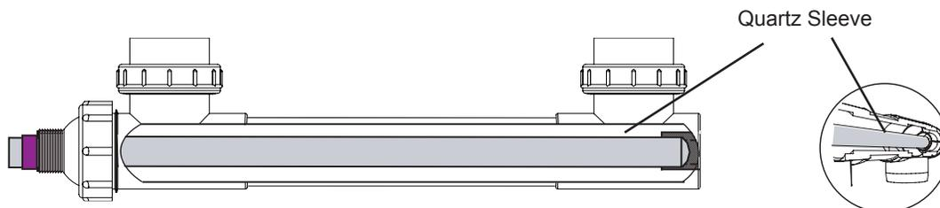
9. Screw on the E-Z Twist Top. Do not use a pipe wrench, pliers or any other tool on this unit. Tighten by hand only. Re-install the Lamp as Shown on page 21, starting at #6.
