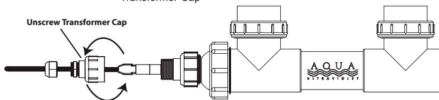
4. Slide Lamp out, be careful not to slide the Lamp out at an angle, even a slight angle, this may cause a "U" shaped crack at the end of the Quartz Sleeve, or possible breakage of the Lamp. Set the lamp on a secure level surface to avoid breakage.
