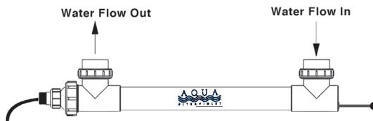
On Wiper Option UV's water should flow into the unit through the opening nearest the end with the wiper ball. This will help ensure that the chamber stays full and the Wiper Rod will not push out.
