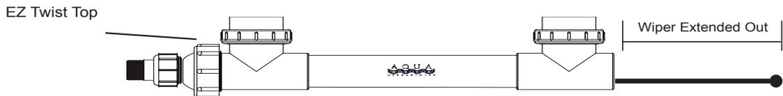
7. Twist off the large cap (EZ twist top) this will release the Quartz Sleeve and the assembly will still be intact.
