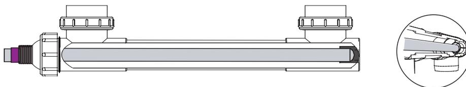
6. Gently push the Quartz Sleeve and Rubber Seal in to the E-Z Twist Top until only 1/2 the rubber seal is visible.
