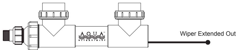
Note: If you have the Wiper option, pull the Wiper Rod out to be fully extended.
