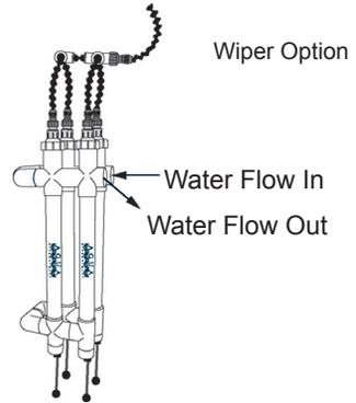
The above are suggestions, if these are inconvenient, either port can be used as the inlet or the outlet. For any installation it is important that the pump flow enough water to keep the UV chamber full; a partially filled chamber allows the seals to dry out including the wiper nut seal on wiper models.
