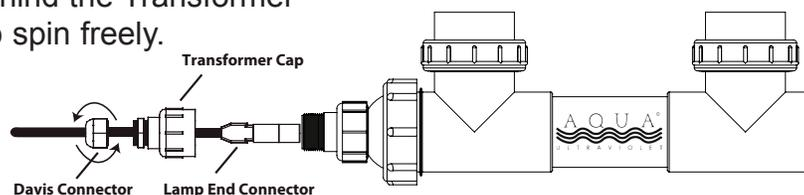
2. Plug the Lamp flush into the Lamp End Connector before inserting the Lamp into the unit. If the Lamp is not plugged in all the way it may cause damage to the unit and is not covered under warranty.
