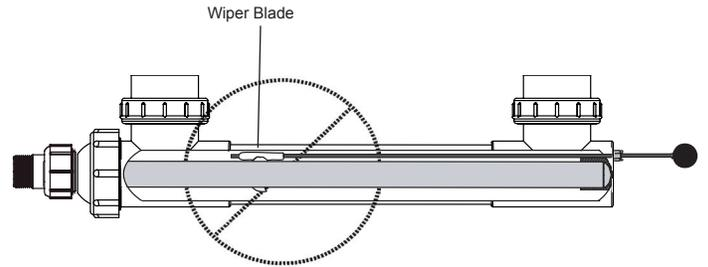
Incorrect: Rubber Seal is Outside of Quartz Cap
