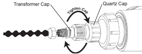
5. Tighten the Hubl Connector back onto the transformer cap.
