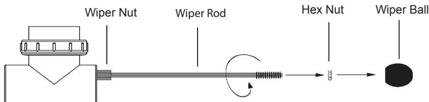
10. Using a 1/2" wrench, unscrew and remove the wiper nut located at the base of the unit. Be very careful not to cross thread.
