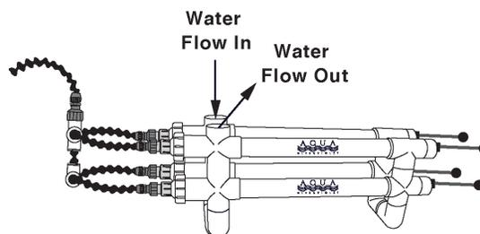
The above are suggestions, if these are inconvenient, either port can be used as the inlet or the outlet. In any installation the pump must be of a sufficient power to keep the chamber full of water so the seals around the wiper nut do not dry out.
