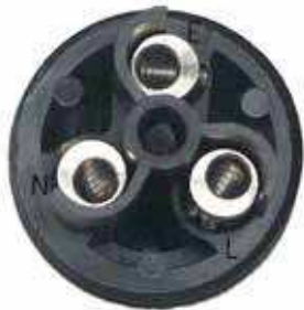
i Figure 5: Wire Connections Brown wire to terminal L Blue wire to terminal N Green/Yellow wire to terminal E
