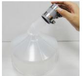
3. Use a slotted screwdriver to tighten on two hose clamps.
