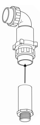
end of the discharge pipe with PVC cleaner/ primer. Apply PVC glue and insert the discharge pipe into the 2" socket fitting. Hold the discharge pipe firmly in place for a few seconds, giving the glue time to set up.
