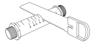
Use a small piece of sandpaper to smooth out the cut end of the discharge pipe. Clean the 2" socket fitting on the bottom of the check valve and the cut
