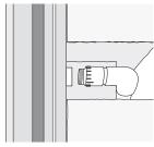
spillway should be tested for proper operation when the wall construction allows. Before final wall installation and covering the basin with rock, the proper flow of the water fall should be adjusted (if needed) with the ball valve.
