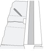
be required for longer spillways or in walls that would require additional weight bearing support. The spillway should be "dry fit" to ensure the spillway is level from side to side and front to back.
